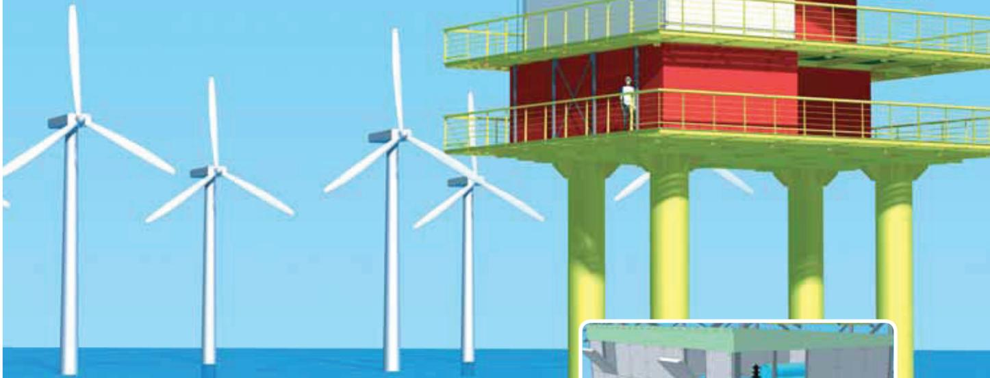
The SCS design team understands the hazardous environment offshore and has learned to design for this harsh environment - inclement weather - wide temperature range - relentless salt spray and corrosion risk throughout the platform's life - typically 30 years. In addition pollution prevention is high on the list of risk mitigation.
